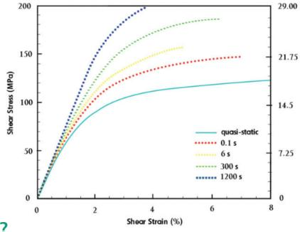
Shear stress-strain response of 45° off-axis specimens at different strain rates <sup>1</sup>
