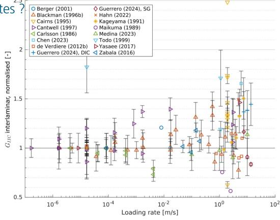
Normalized mode II ERR for various UD-reinforced CFRP materials from quasi-static to dynamic loading rates<sup>2</sup>
